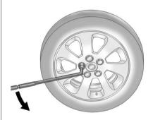
Use the wrench to loosen all the wheel nuts. Do not remove them yet.
